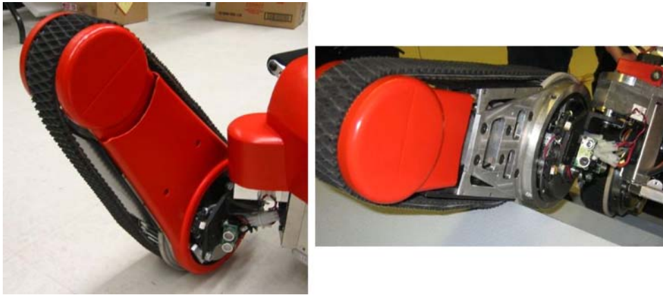
Figure 17. Closer views of the articulations on the floor (left) and on stairs (right).
