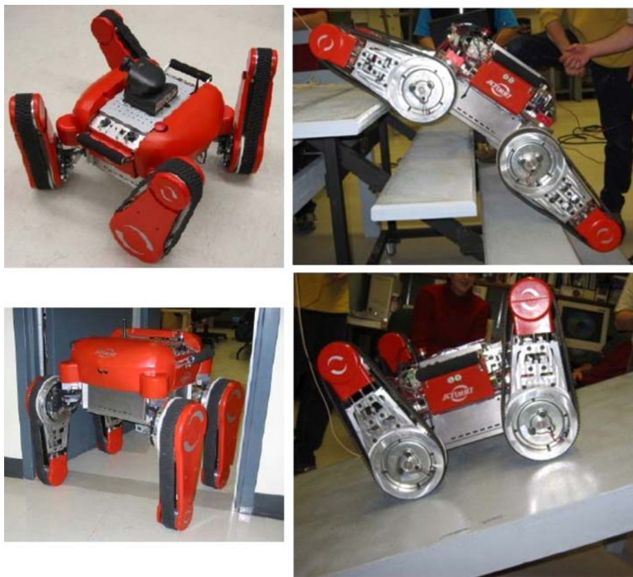
Figure 15. AZIMUT with its articulations in different positions (top left), on stairs (top right), going through a door (bottom left), and on an inclined surface (bottom right).
