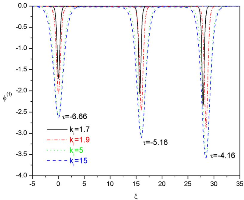
**Fig. 2** Time evolution of cylindrical solitary waves,  $\phi^{(1)}$  versus spatial coordinate  $\xi$  at times  $\tau = -6.66$ ,  $\tau = -5.16$ , and  $\tau = -4.16$  for  $\sigma = 0.1$ ,  $\mu = 0.1$ ,  $k_i = 3$  and different values of  $k_e$
