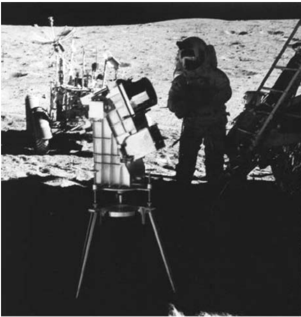
Fig. 3 The S201 experiment on the lunar surface, deployed in the shadow of the Lunar Excursion Module of the Apollo 16 mission (source: NASA)
