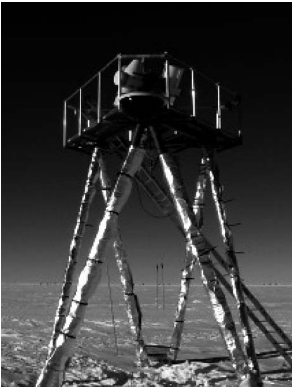
Fig. 1 An Antarctic telescope, such as the AFOS (Antarctic Fibre Optic Spectrometer), has to operate high above the icy surface to prevent built-up of wind-blown snow and to reach atmospheric levels with excellent seeing (source: Dempsey et al. 2004)
