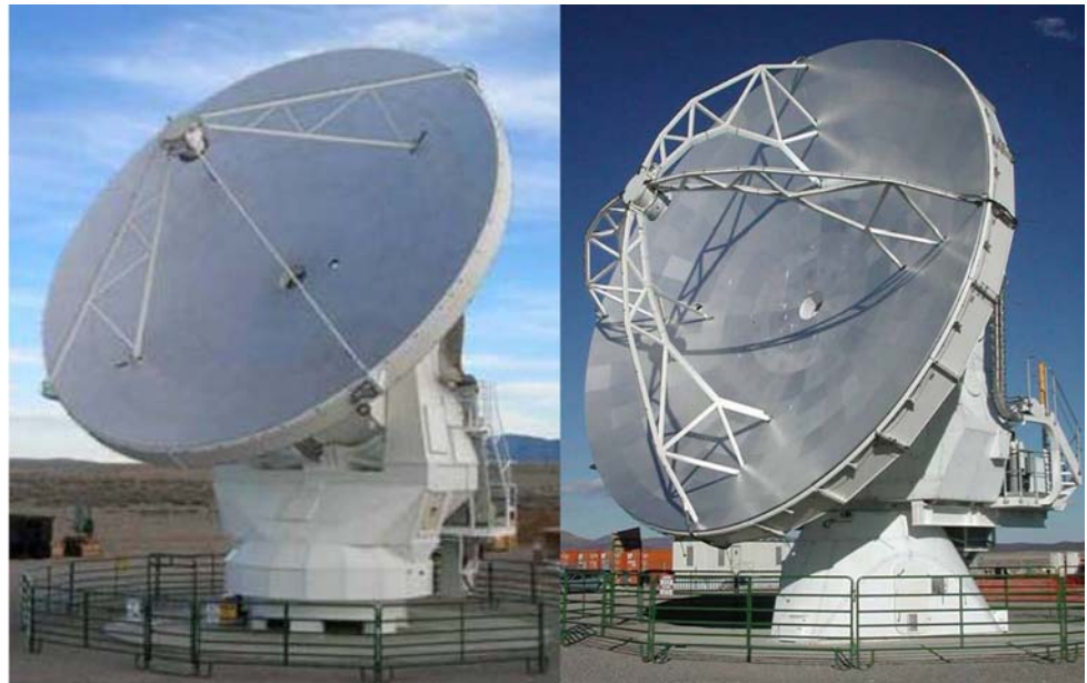
Fig. 5 The Alcatel ( left ) and Vertex ( right ) antenna prototypes, built at the VLA site in New Mexico
