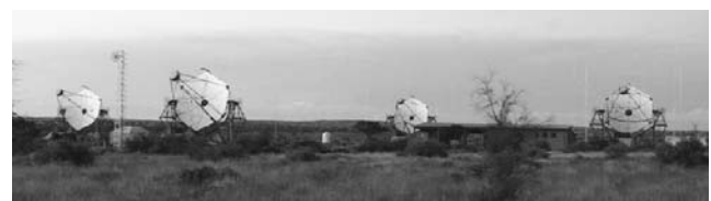
Fig. 1 The HESS array of 4 imaging atmospheric Cherenkov telescopes located in Namibia at 1 800 m a.s.l.
