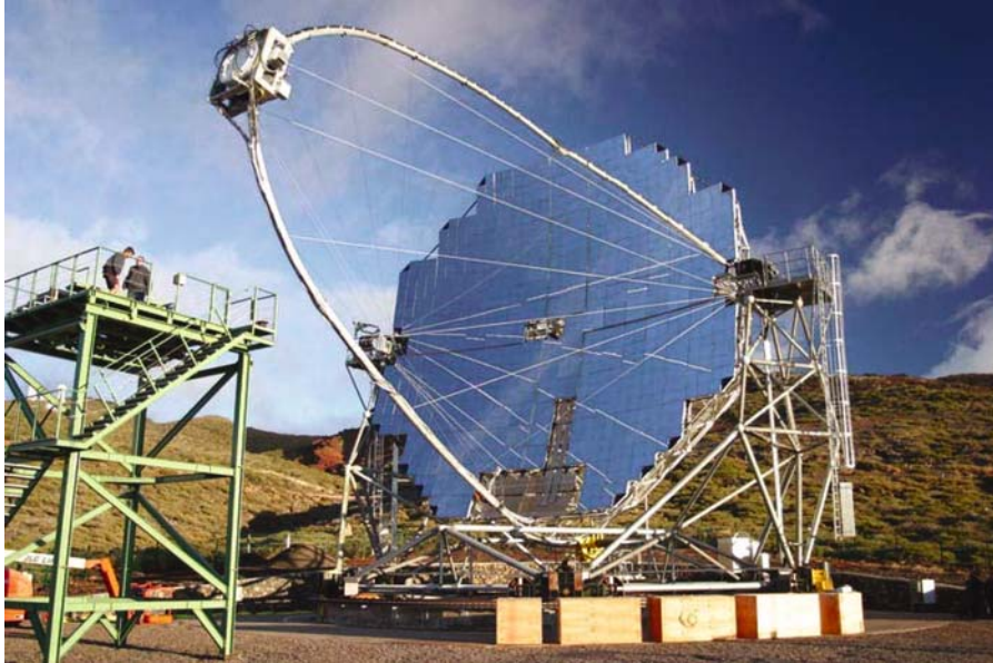
Figure 1. View of the MAGIC telescope just before its inauguration in October 2003. Its 17 m diameter reflector makes it the largest Imaging Cherenkov Telescope in the world. The main mirror is composed of 940, 1 m 2 mirror panels that are fully steerable using an active mirror control system.
