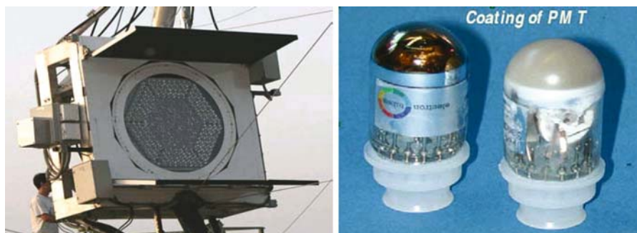
Figure 2. On the left a view of the telescope camera with its 577 PMTs. The inner section of the camera is made up of 397 0.1^\circ field-of-view pixels, surrounded by four rings of 0.2^\circ pixels. The second picture shows two Electron Tubes PMTs. The “frosted” PMT on the right has been coated with a wavelength shifter lacquer that increases the quantum efficiency by 30% (coating all the PMTs is roughly equivalent to increasing the mirror area from 240 to 300 \text{m}^2 ).
