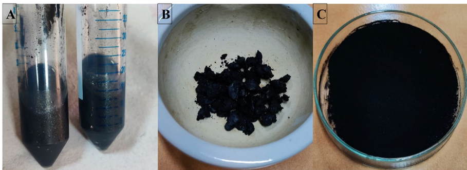
Fig. 2 The extraction of squid ink using n-hexane (a), dried form of squid ink (b), and fine powder sieved in 150- \mu mesh (c)
