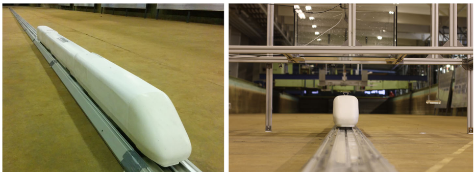
Fig. 2 Model (simple configuration) in empty towing tank
