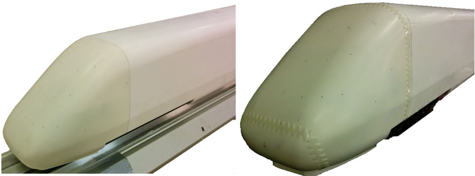
Fig. 3 First car with (right) and without (left) tripping tape (12 mm × 0.4 mm)
