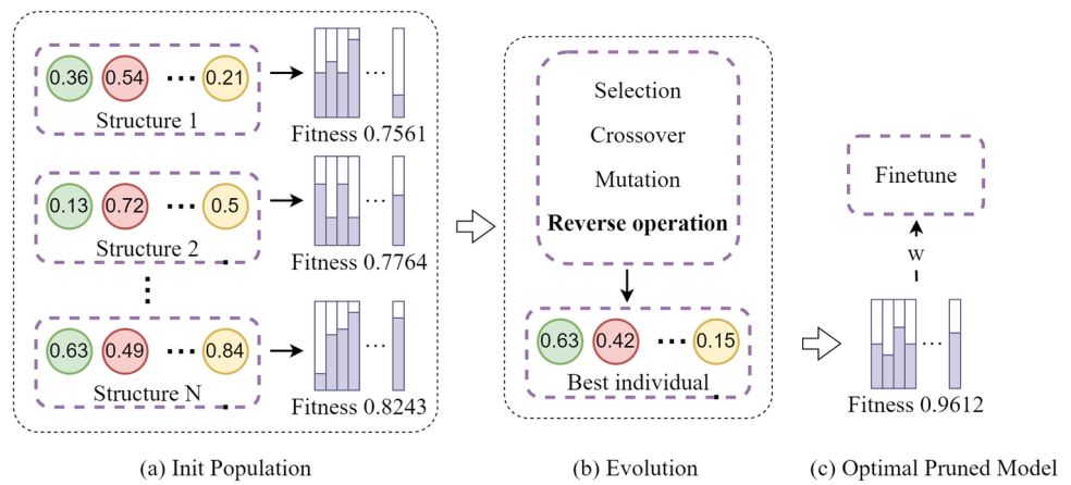
Fig. 2 AFPruner algorithm framework. The optimal pruned model is obtained through genetic algorithm, and then fine-tune to recover the model accuracy
