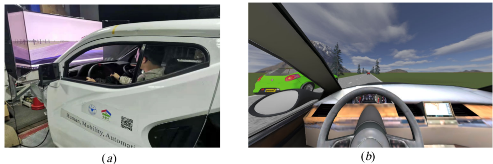
Fig. 3 (a) The 6-DoF driving simulator. (b) Lane change scenario in Prescan
