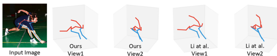
Fig. 1 Comparison with the visual results of Li et al. [23] on the MPI-INF-3DHP dataset. We obtained more accurate recognition results (legs etc., for view 2)
