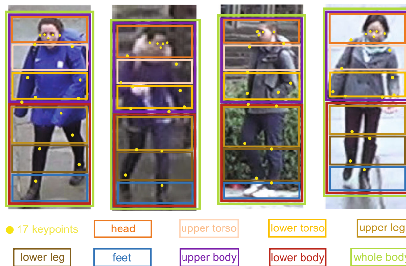
Fig. 5 Examples with 17 keypoints and nine part partitions. We used OpenPose [26], which was pretrained on the MS COCO2017 dataset [41], to obtain the coordinates of 18 keypoints in the original image, including 'nose', 'neck', 'right shoulder', 'right elbow', 'right wrist', 'left shoulder', 'left elbow', 'left wrist', 'right hip', 'right knee', 'right ankle', 'left hip', 'left knee', 'left ankle', 'right eye', 'left eye', 'right ear', and 'left ear'. According to our experience, when applying the pretrained model to Re-ID datasets, the estimation of 'neck' has a large deviation. Therefore, we removed 'neck' but retained the remaining 17 keypoints. The yellow dots in each image represent the 17
