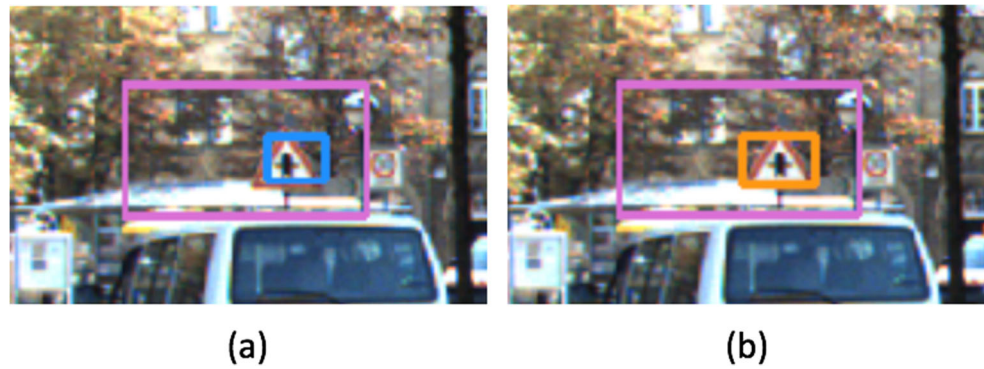
Fig. 10 A traffic sign example in Seq. 0005 from KITTI, showing proposal box with regressed box. a Proposal box in blue color; b Regressed box in orange color. Pink rectangle denotes the promising region for proposal selection
