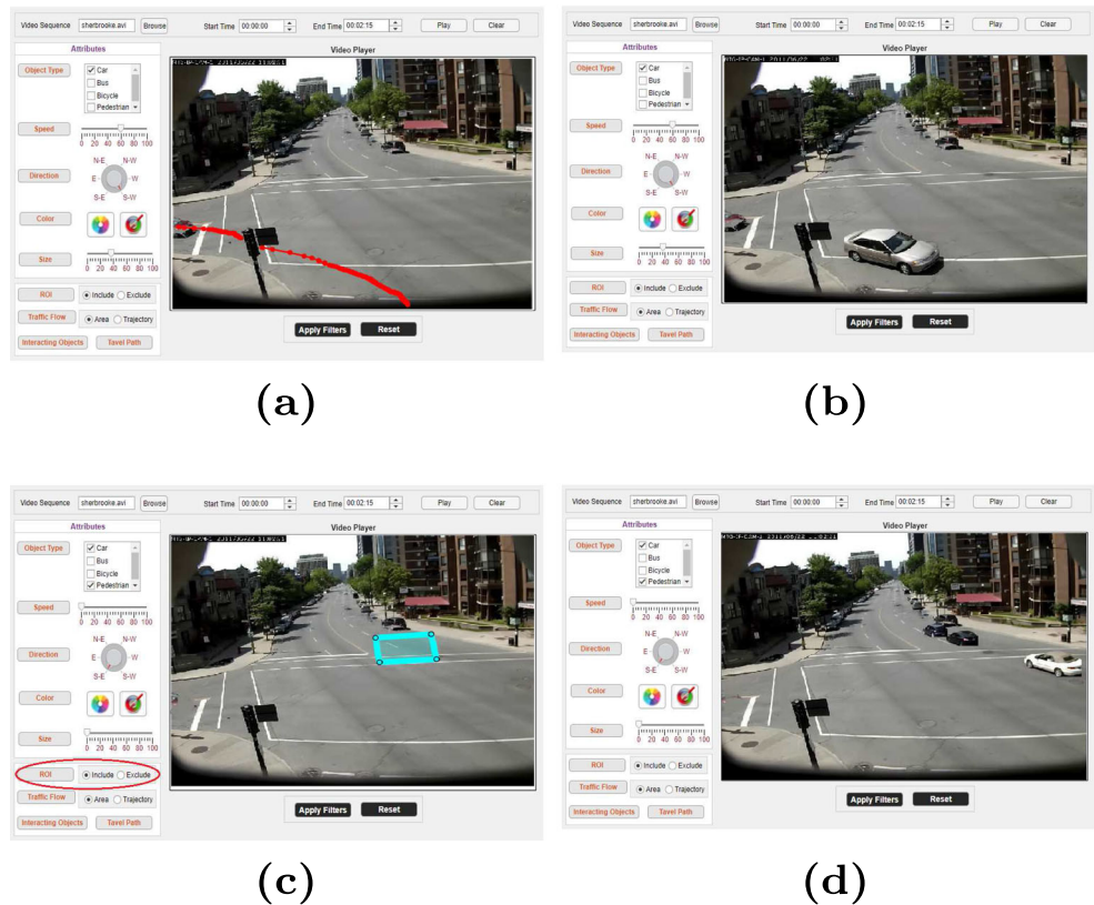
Fig. 4 Sample spatial query a Activity path of interest (shown in red color) drawn on a video frame by a user. b Sample frame from the corresponding synopsis video. c ROI (see the rectangle) marked to include tubes in the synopsis video. d Sample frame from the corresponding result
