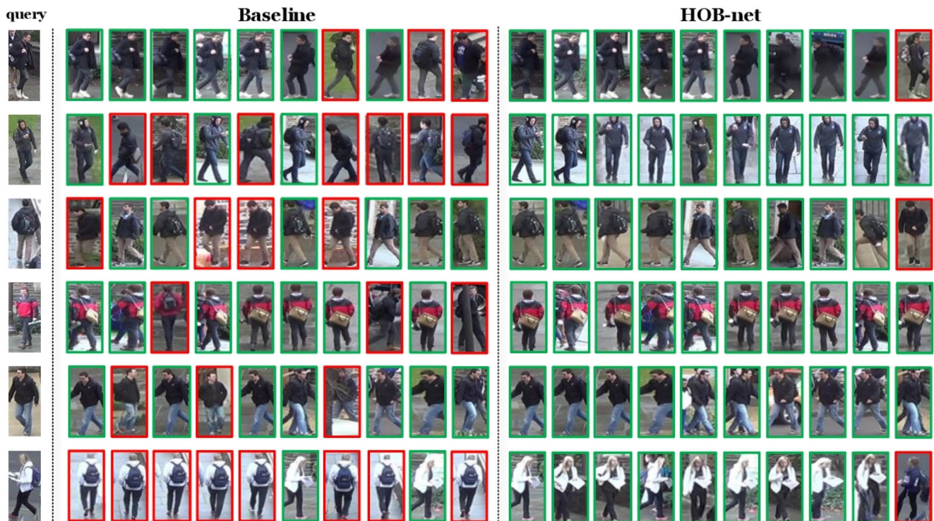
Fig. 9 Example results of six query images on DukeMTMC-ReID. Each row shows the top-10 retrieved images of Baseline and HOB-net. Person surrounded by green box denotes the same person as the query image, the red one is different
