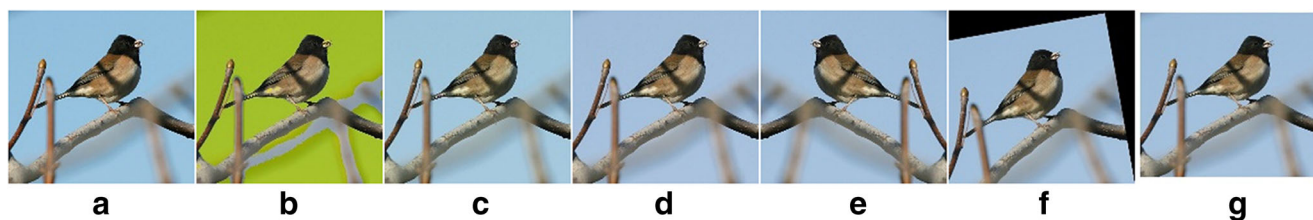
Fig. 2 Image data augmentation. a Original image, b Hue Shift, c Saturation Shift, d Brightness Shift, e Mirror Flip [35], f Rotation, g Random Padding [36]
