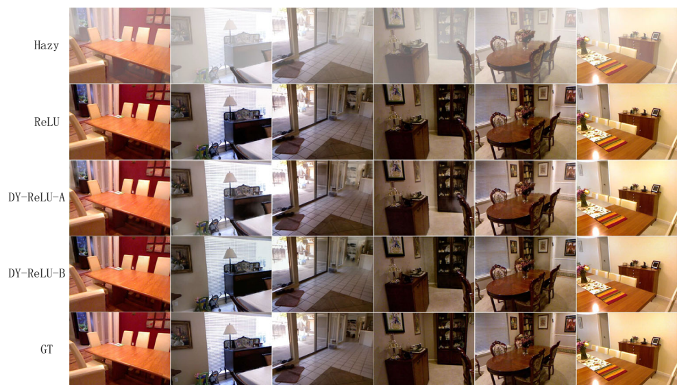
Fig. 6 Selection of test results using different activation functions for the outdoor synthetic image dataset
