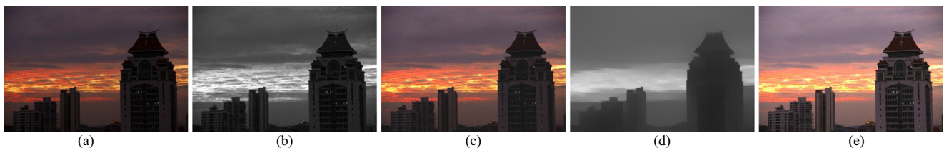
Fig. 4 Illumination estimation. a Input image. b Initial illumination. c Result recovered from (b) . e Result recovered from (d)
