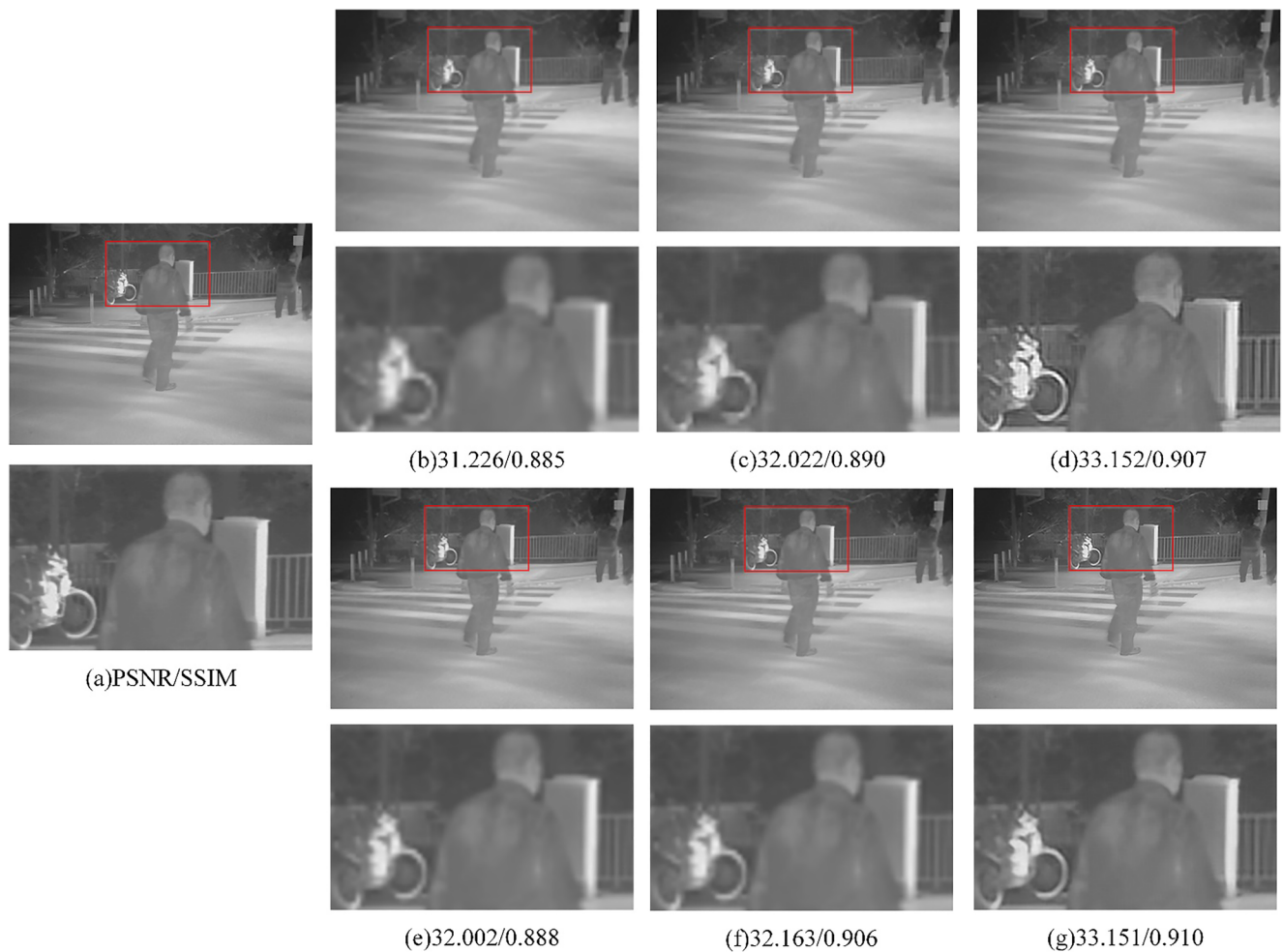
Fig. 7 Visual result comparison of various methods and the proposed model on Test2-people with an upscaling factor of 4. (a) Ground-truth HR; (b) Bicubic interpolation; (c) SRCNN; (d) DRCN; (e) SRGAN; (f) ESRGAN; and (g) Ours
