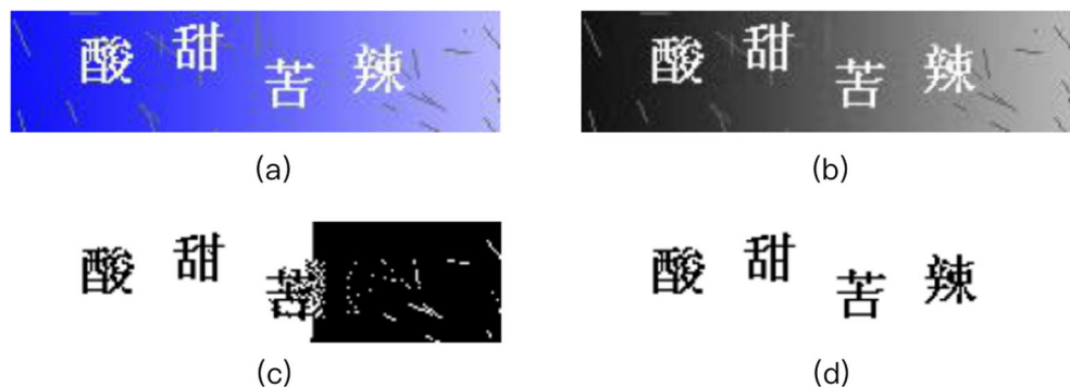
Fig. 4 Usage of morphological reconstruction on an CAPTCHA image with gradient background color. a Original image; b Grayscale image; c Binarized image; d Binarized image with morphological reconstruction
