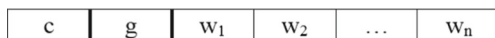
Fig. 3 The structure of a chromosome for optimizing C , \gamma and weights of features
