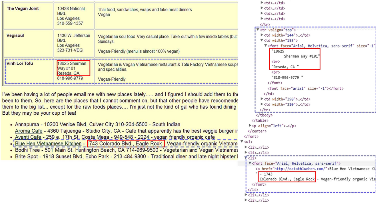
Fig. 6 Two address layouts in a webpage and the corresponding HTML codes (the red blocks denote the detected addresses and the blue dashed blocks denote the corresponding associated information). Such multi-list layout can not be handled by Chang and Li’s method which treats just one record pattern
