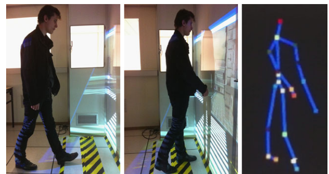
Fig. 17 Kinect "Move:Walk" event detection
