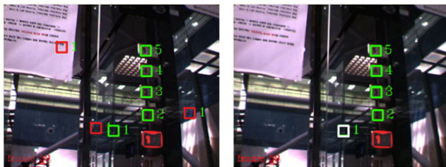
Fig. 14 False positives arising from an imperfect outlier rejection at frame 59 in a non-retrained case. The white square in the right image is falsely-recognized button
