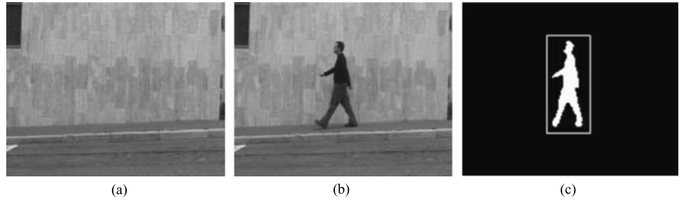
Fig. 2 (a) Background image, (b) Frame from a walking sequence, and (c) ROI within a rectangle
