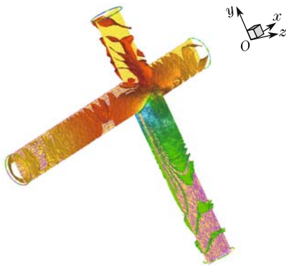
Fig. 4 Calculating chart of 3D isobaric surfaces and centre-sectional velocity vectors of USGA nozzle
