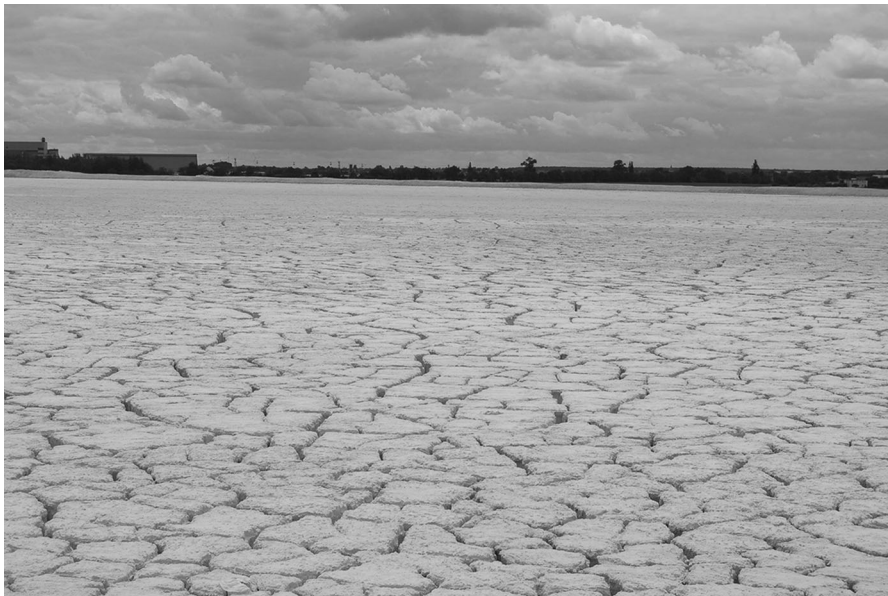
Fig. 1 The surface of the saline soda lime deposited in the repository in Janikowo
