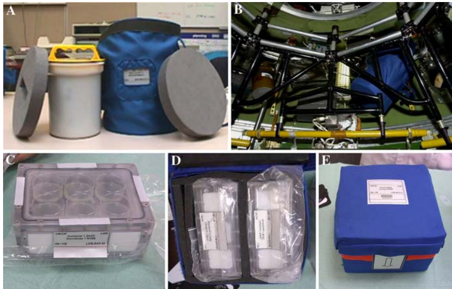
Fig. 1 Spaceflight experiments hardware. a The hardware used for the spaceflight experiments MESSAGE-1 and -2 was composed of basic commercially available standard sterile laboratory plastic components. c, d, e For the BASE-A spaceflight experiment a special transparent Biocontainer was constructed allowing manual in-flight photography of the
