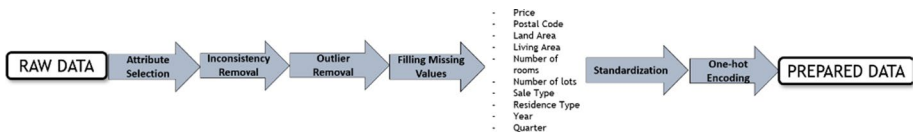
Fig. 7 Main steps of data preparation without geocoding
