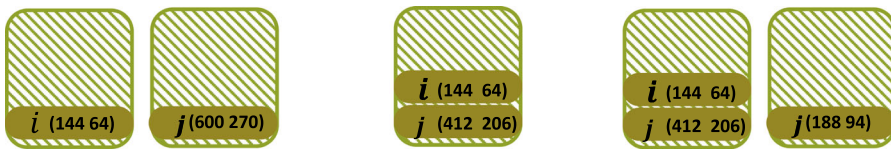
Fig. 3 Three loading scenarios: Scenario One—Start loading the current order j onto an empty pallet. Scenario Two—Start loading the current order j onto the same pallet as the previous order i (order j can be completely loaded.). Scenario Three—Start loading the current order j onto the same pallet as the previous order i (order j can be partially loaded)
