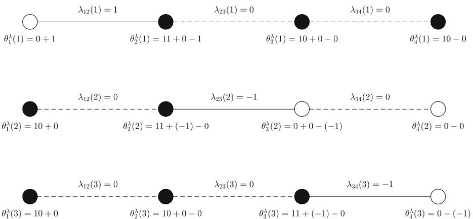
**Fig. 1** An example of an interior local minimum of the Potts problem, non-zero  $\lambda$  variables are denoted by solid lines and zero  $\lambda$  variables are denoted by dashed lines. All values should be halved, which was omitted for clarity and better reading
