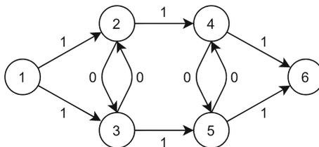
**Fig. 3** Directed graph with 6 nodes, 10 edges,  $s = 1, t = 6$ , and edge weights from the set  $\{0, 1\}$  (indicated next to the edges). Dual feasible solution  $y = (4, 3, 3, 1, 1, 0)$  is an interior local maximum of (40) with objective 2 but not a global optimum, which has value 3. The vertex indices are indicated by the numbers within the corresponding circles
