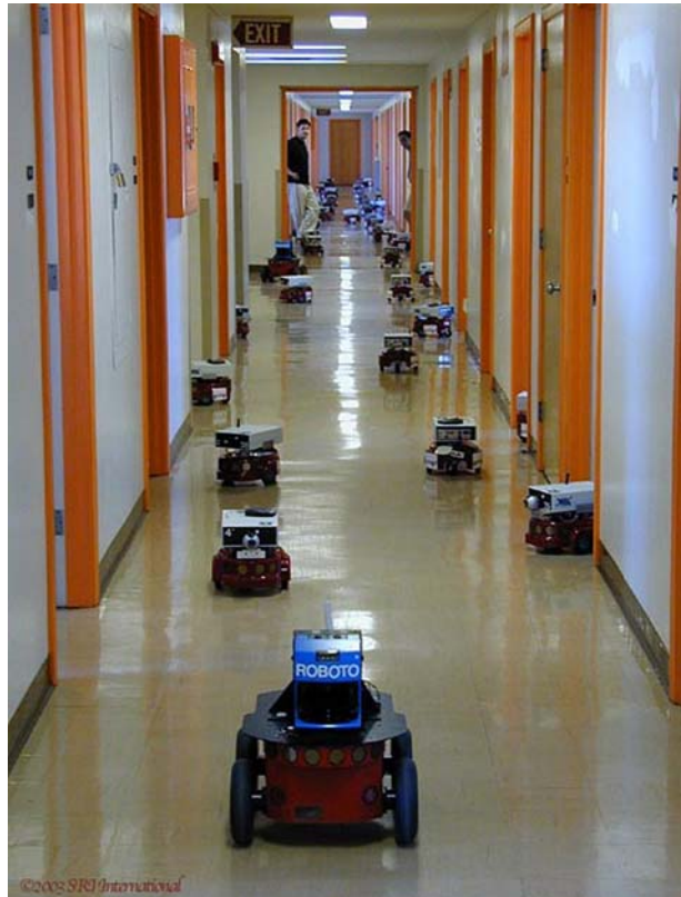
Fig. 1 CentiBots development and evaluation team. The four larger robots in the back, Pioneer IIs with SICK laser range-finders, are used for mapping and exploration. The rest are Amigobots with sonars, a camera and a small PC on top
