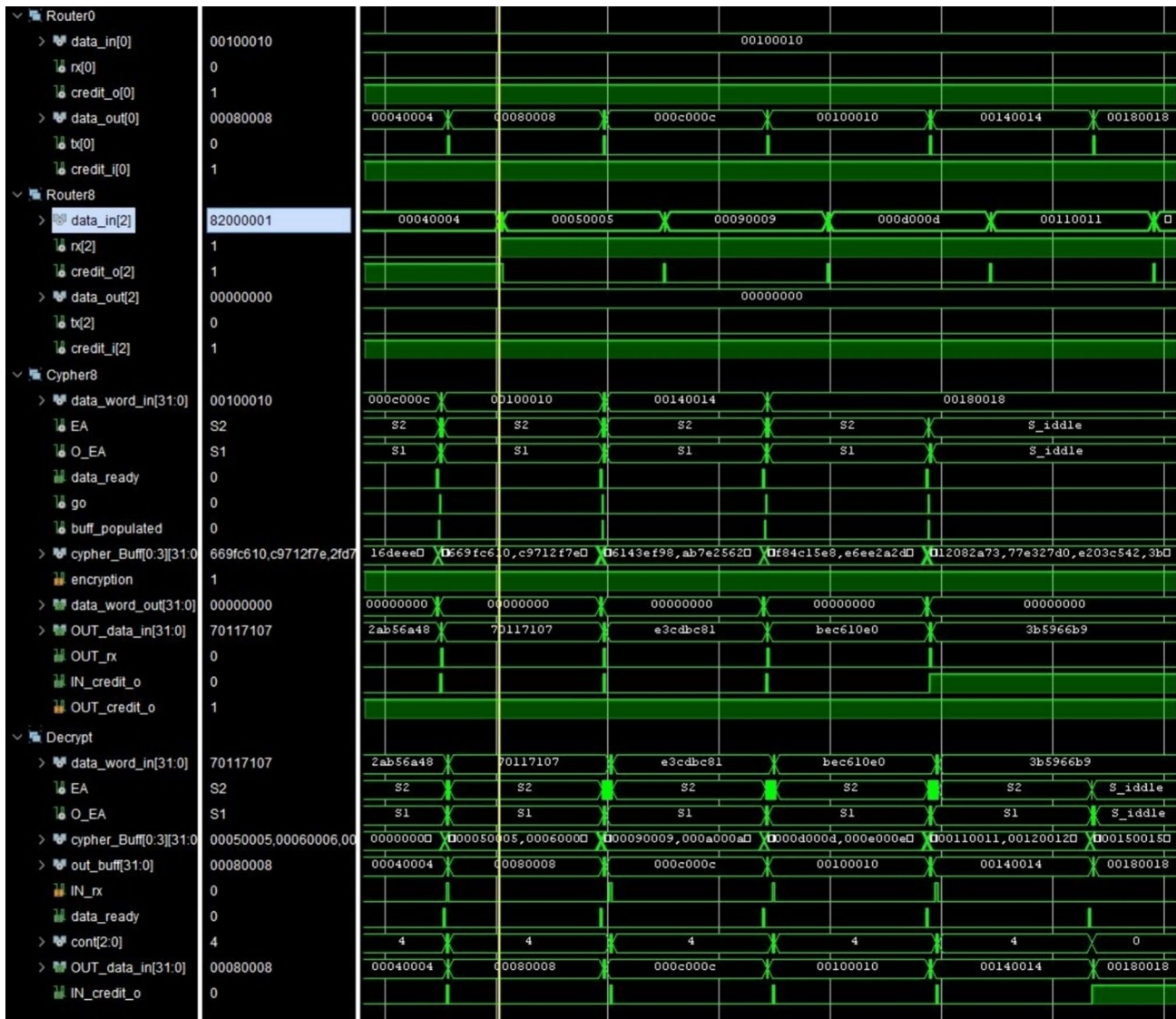
Fig. 7 ILA simulation results of proposed NoC architecture in Zynq-SoC
