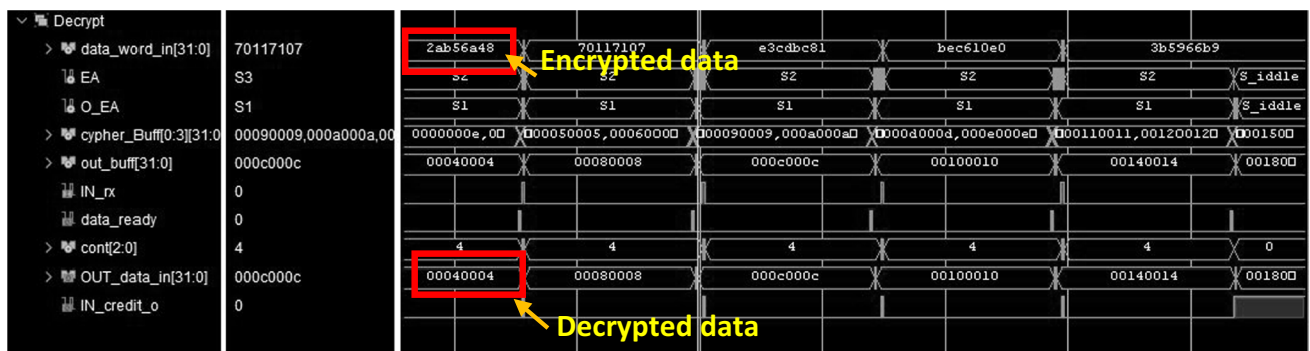
Fig. 6 The Decryption simulation results
