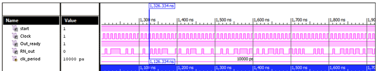
Fig. 7 Outputs of Elliott-93 approach based PRNG
