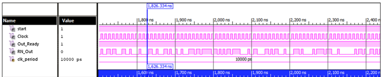
Fig. 6 Outputs of TS-5 approach based PRNG
