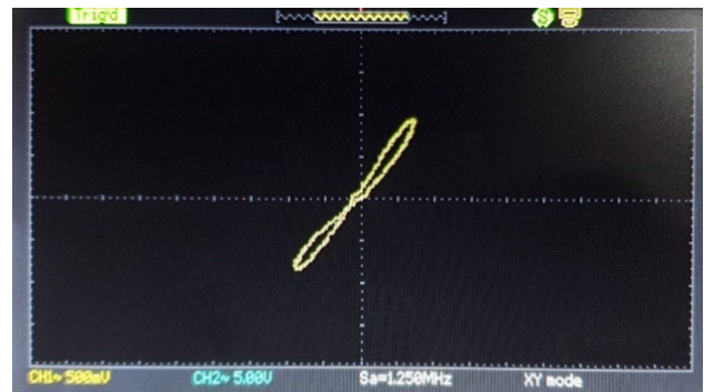
Fig. 12 Pinched Hysteresis loop of experimentally realized proposed memristor emulator circuit observed on CRO
