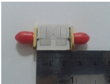
Fig. 15 Photograph of the fabricated proposed filter
