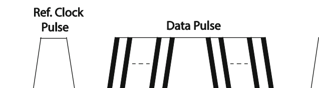
Fig. 2 The timing diagram of the DTR-DTS transmitted signal
