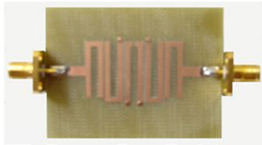
Fig. 13 Snap shot of filter on FR4 ( \epsilon_r = 4.34 )
