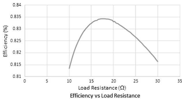
Fig. 9 The relation between efficiency and R_L
