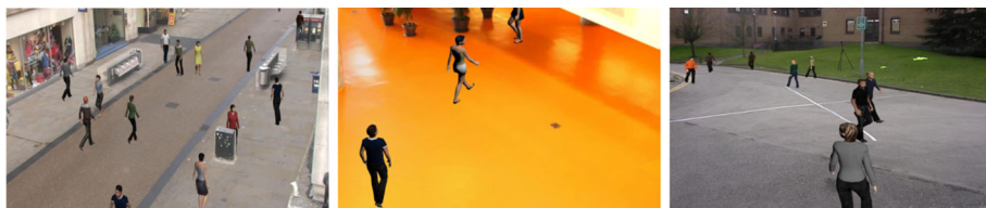
Fig. 12 Constructing artificial scenes by superimposing virtual pedestrians onto the real background images
