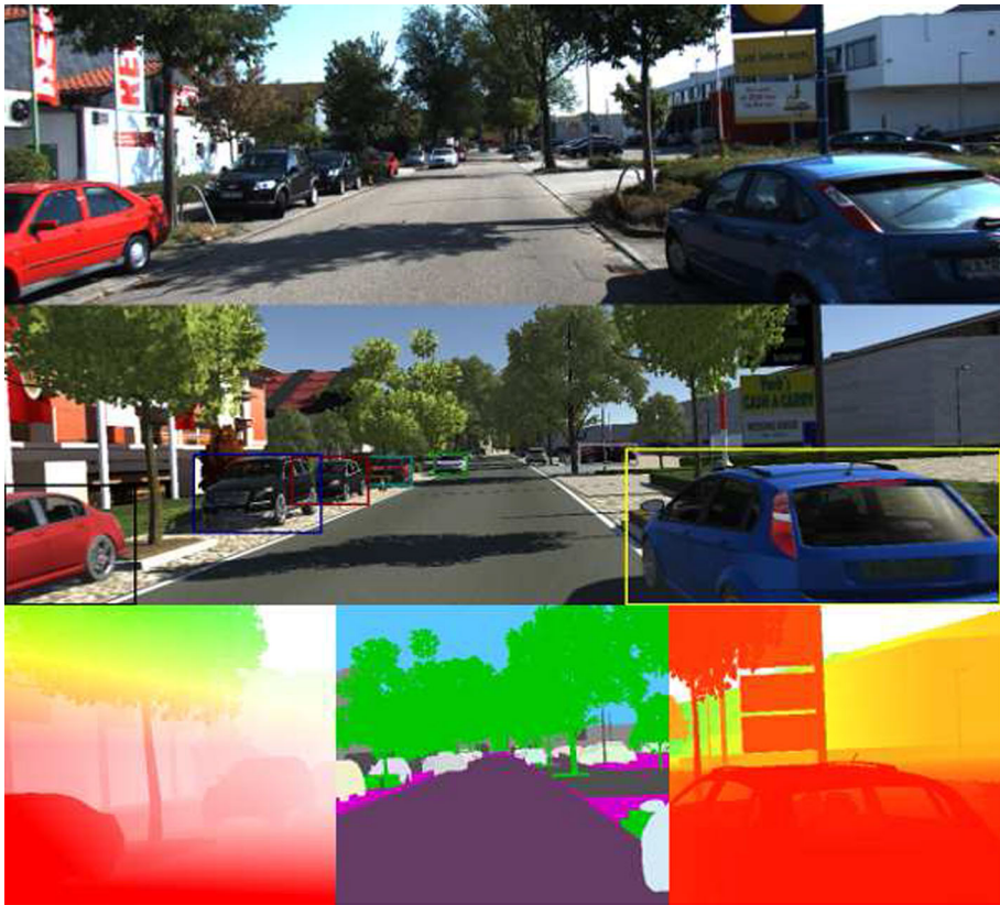
Fig. 5 The Virtual KITTI dataset (Gaidon et al. 2016). Top : a frame of a video from the KITTI multi-object tracking benchmark. Middle : the corresponding synthetic frame from the Virtual KITTI dataset with automatic tracking ground truth bounding boxes. Bottom : automatically generated ground truth for optical flow ( left ), semantic segmentation ( middle ), and depth ( right )
