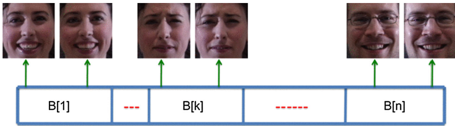
Fig. 1 The dictionary has a block structure where the training images of each subject form a few blocks
