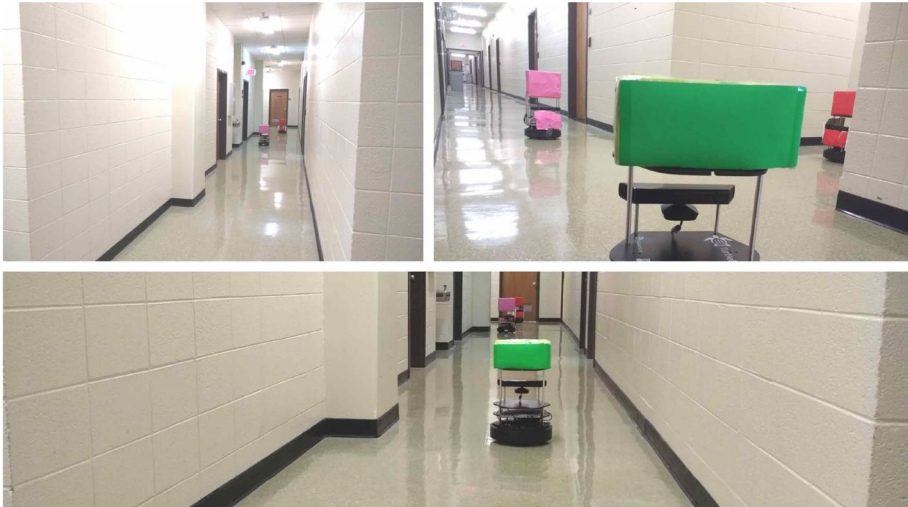
Fig. 4 (top-left) Patrollers (in pink and red) in the longer hallway of instance 2 of the domain. (top-right) Learner's (green) perspective as it observes the patrollers from its vantage point. (bottom) Learner penetrating the patrol to reach the goal undetected (first door on its right). The learner perceives the location and the orientation of each patroller by using the depth and the bounding box for the color blob detected via CMVision.
