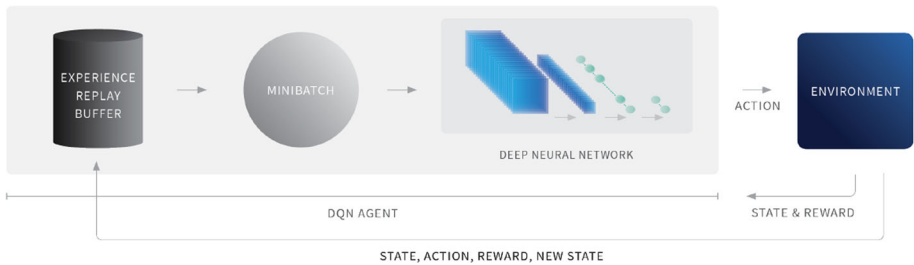
Fig. 3 Representation of a DQN agent that uses an experience replay buffer [193,194] to keep \langle s, a, r, s' \rangle tuples for minibatch updates. The Q-values are parameterized with a NN and a policy is obtained by selecting (greedily) over those at every timestep
