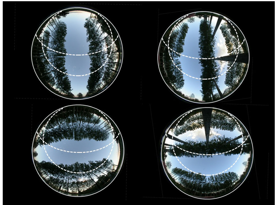
Fig. 4 Sun path during the summer solstice at 25° and 65° of latitude North between North–South (top) and East–West (bottom) oriented tree lines, as seen from the centre of the cropped alley (left) or close to the tree line (right). Picture shot in a poplar alley cropping system with tree lines spaced 16 m and tree height 20 m. At 65° of latitude North, the sun path is almost a full circle
