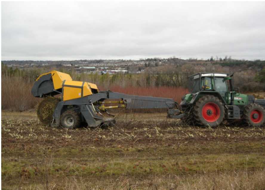
Fig. 4 Anderson biobaler harvester being operated by a 100 kW tractor, GARS, Guelph, Ontario, Canada
