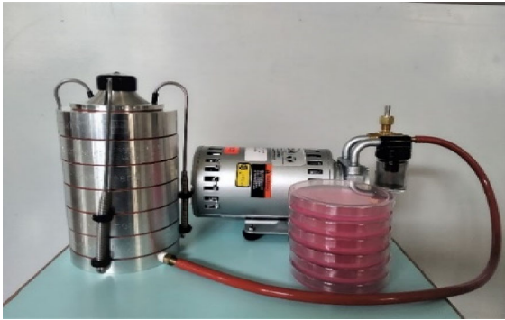
Fig. 2 Anderson Six stage Bioaerosol Impactor used for air sampling
