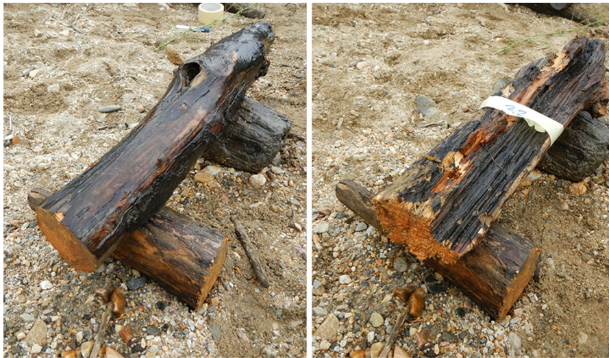
Fig. 6 Example of fresh (left) and rotten logs (right) installed at the Lafnitz River
