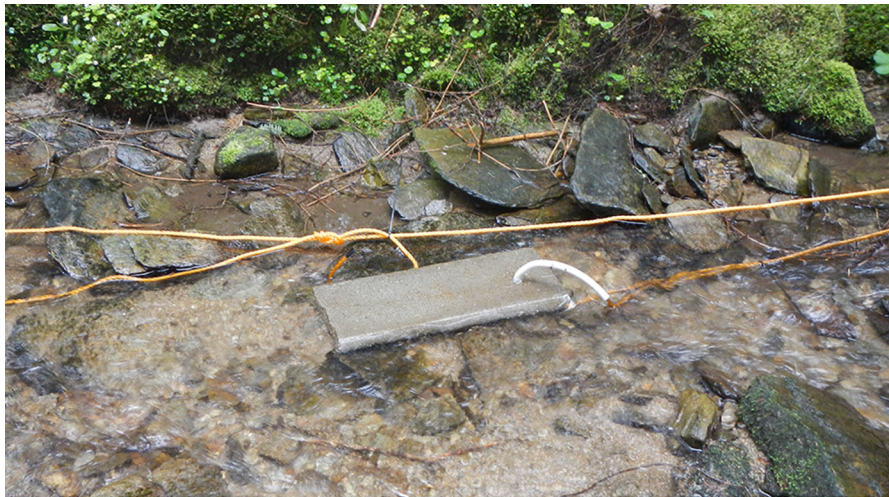
Fig. 5 Example of one installed concrete bar at site A
