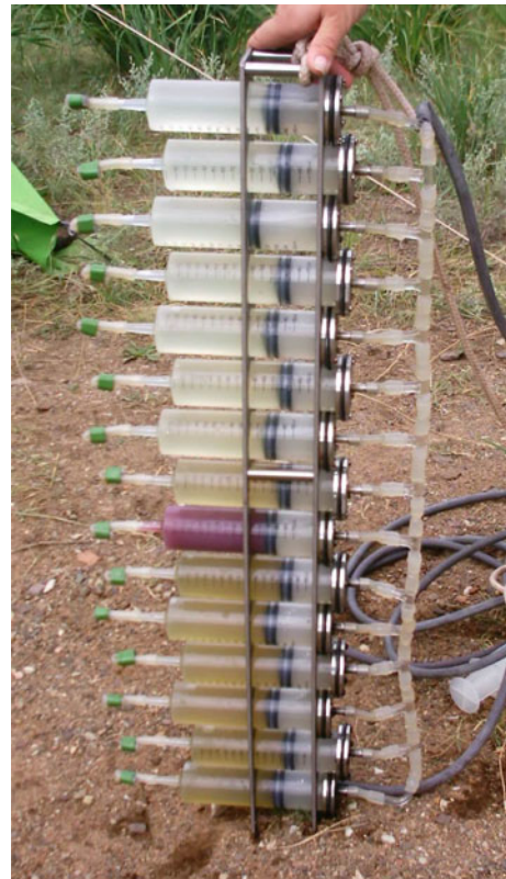
Fig. 1 Multi-syringe thin-layer sampler (Rogozin and Degermendzhy 2008). The photo shows 15 simultaneous, vertical samples taken from Lake Shunet (Siberia, Russia) in August 2004 at 5-cm intervals. The “purple layer” can be easily distinguished (the 9th syringe from the top)
