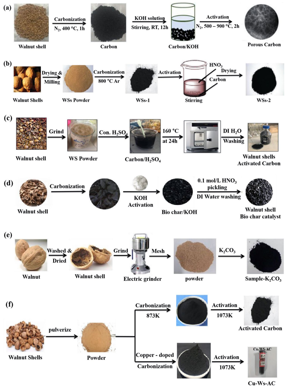
Fig. 1 Different types of CA processes of WS. (a) KOH activation [42], (b) HNO 3 activation [47], (c) Con. H 2 SO 4 activation [48], (d) KOH activation [43], (e) K 2 CO 3 activation [44], and (f) KOH activation [45]
