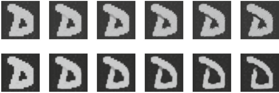
Fig. 1 Morphing of letter D from MNIST training set: top row shows evolution of the template; bottom row shows evolution of deformed template
